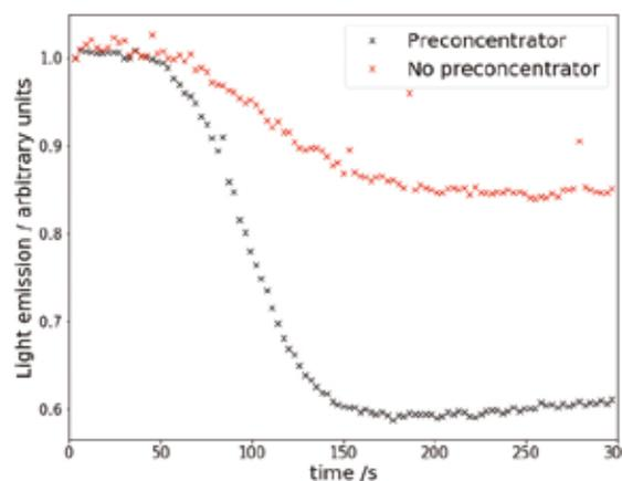
Figure 2: Response of a super yellow thin film sensors exposed to silicon wafers that have previously been exposed to DNT contaminated nitrogen. The wafers are heated to 100°C in a sealed chamber with the sensor, and the light emission of the sensor is monitored. The red trace is the response from a bare silicon wafer and the black trace the response from a Aflas® coated wafer.
